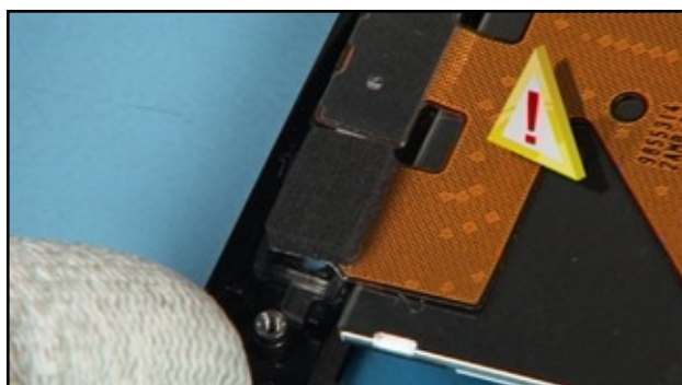
44. Be double carefull while lifting out the CMOS CAMERA MODULE.
